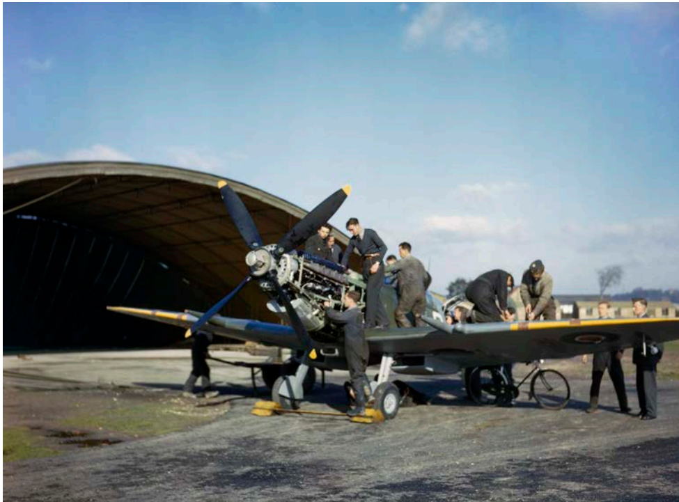
A Spitfire Mk IX of 64 Squadron undergoing an engine overhaul outside a Blister Hangar on the north side of Fairlop.
